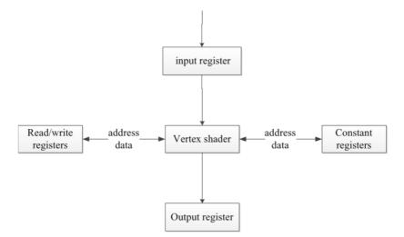
Fig. 2. Structure diagram of vertex shader
